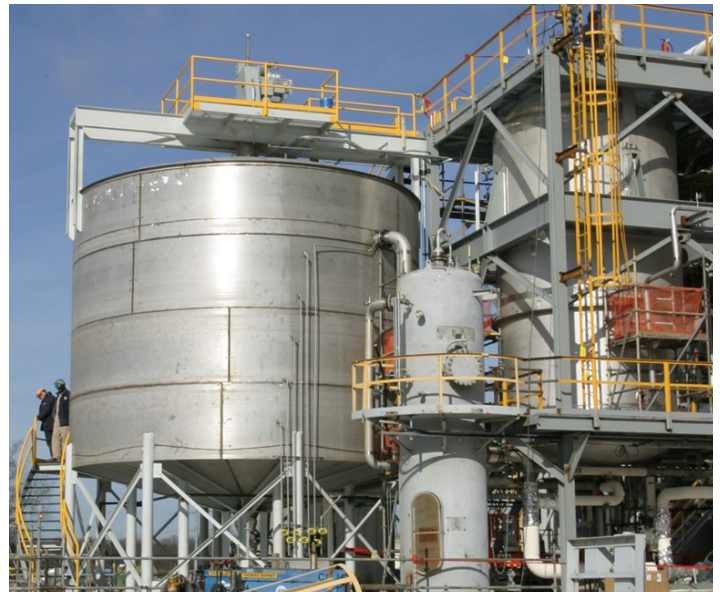
26' Dia 316 ss Custom Shaft Drive with Lift & Elevated 316 ss Covered Tank (With Erection)
